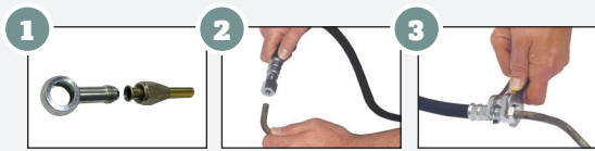
1 Cut tubing to size, flare, install correct fitting from assortment
