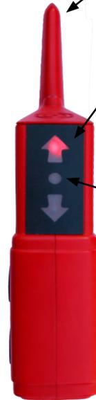
The “Wire Harness Probe” is for probing a harness to detect the open circuit signal. (See “Tracing Circuits that are Shielded” pg.21 )
